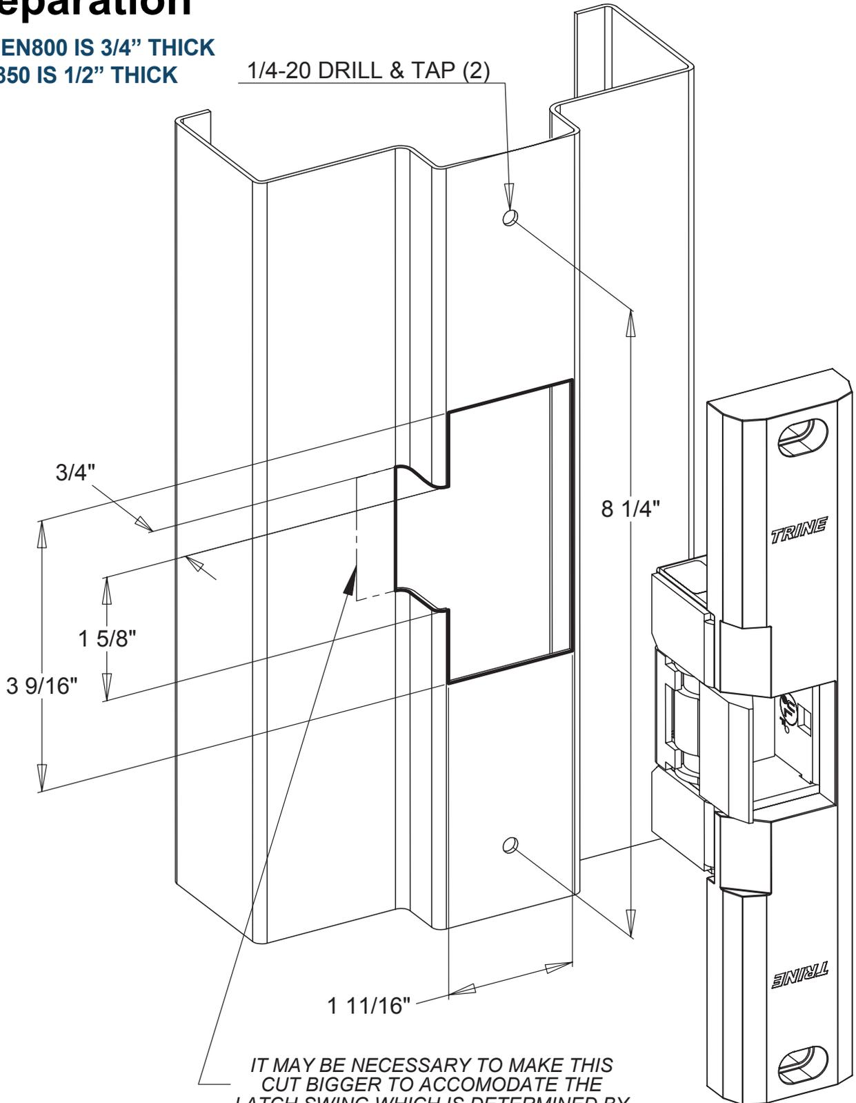
IT MAY BE NECESSARY TO MAKE THIS CUT BIGGER TO ACCOMMODATE THE LATCH SWING WHICH IS DETERMINED BY HOW DEEP THE LOCK EXTENDS INTO THE STRIKE CAVITY.
