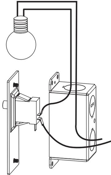
Contact rating- 10 Amps at 120 volts
