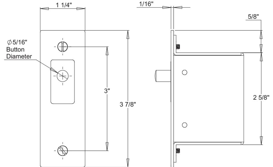
The door switch can be mounted to the switch case with the 2 flat head screws (supplied).
