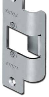
For new or replacement installation in wood or metal frames. Use with cylindrical locksets having up to 5/8" throw, based on 1/8" door gap.
